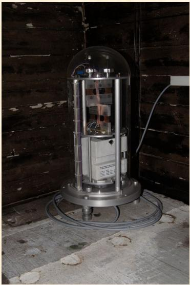
Fluxgate 3-component magnetometer FGE - (Paratunka, Magadan)
