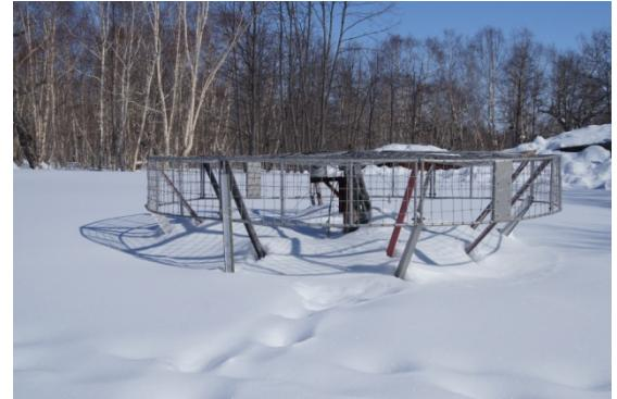
Sensor of vertical gradient of electric field potential “Pole-2” at GFO
